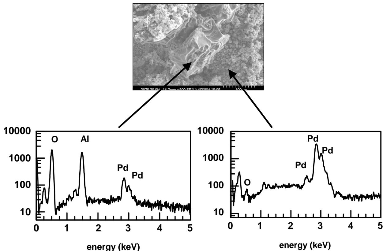
**Figure 5. SEM of Pd/D electrode, after being placed in an external electrostatic field, showing a “boulder-like” deformation. XRF spectra showing the chemical composition of the boulder and the area adjacent to the boulder.**
