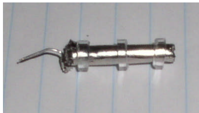
FIGURE 9. Picture of cylinder made using palladium foil.
