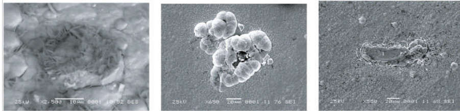
a. Needle formations on the boundary b. Broken cocoon. c. Micro explosion "crater"
