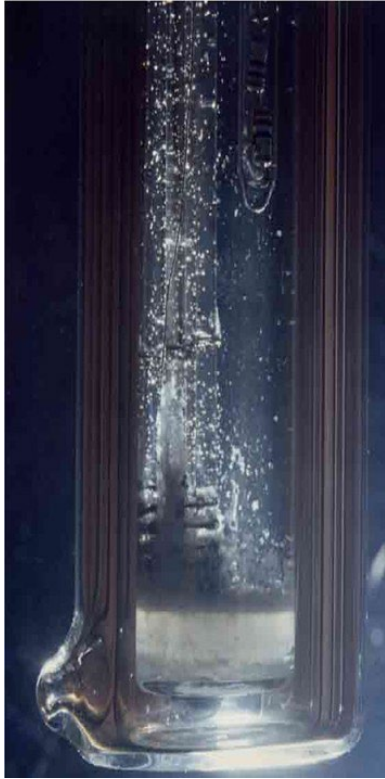
Figure 5. Close up of an Icarus cell undergoing electrolysis in an experiment by Biberian and Lonchampt. Courtesy J.-P. Biberian
