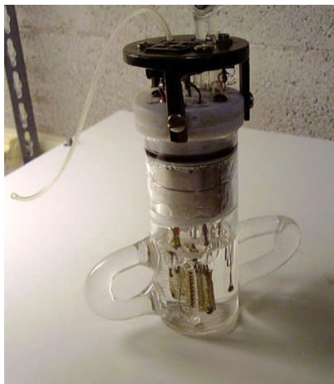
Figure 1. A cell made by E. Storms for a Seebeck calorimeter, with “cooling fins”—tubes extending from the cell filled with electrolyte, which increase surface area. These fins would defeat the purpose with an isoperibolic calorimeter.
