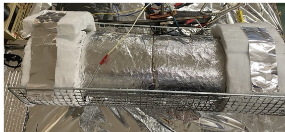
Fig. 7. The entire container was covered with insulation to ensure a uniform temperature.
