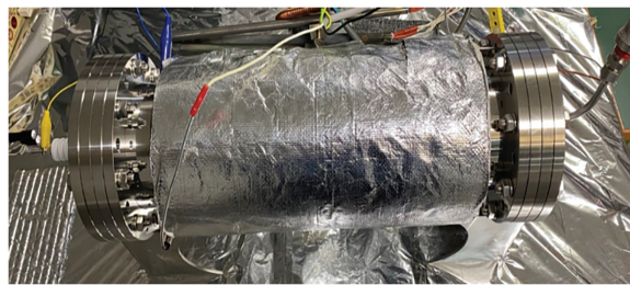
Fig. 6. Container covered with insulating material.
