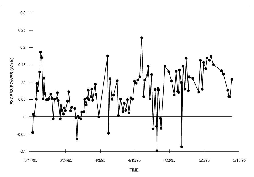
Initial Excess Power For NRL Pd-B Rod (Cell D) (0.25 wt. % B, 0.20 x 2.0)  $V = 0.25 \text{ cm}^3$ , March 1995 – May 1995  $P_x \text{ (max)} = 90 \text{ mW}$
