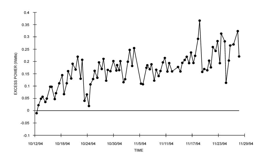
Excess Power For NRL Pd-B Rod (Cell A) (0.50 wt. % B, 0.40 x 2.0 cm, V=0.25 cm³, March 1995-May 1995  $P_X\left(max\right)=150~mW$
