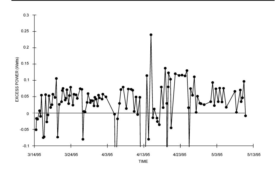
Excess Power For NRL Pd-B Rod (Cell C) (0.25 wt. % B, 0.40 x 2.0 , V=0.25  $cm^3$ , March 1995-May 1995  $P_X(max) = 200 \text{ mW}$
