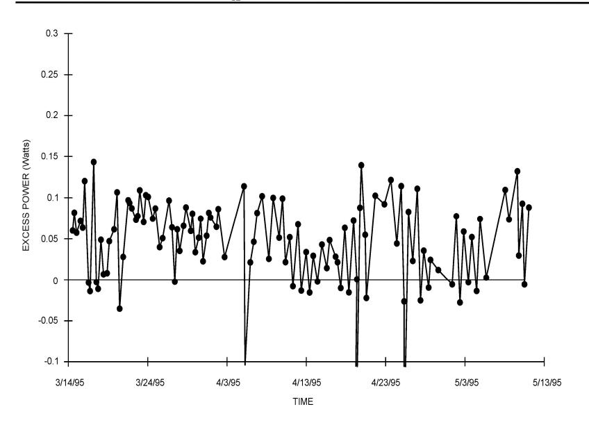
Excess Power For NRL Pd-B Rod (Cell B) (0.50 wt. % B, 0.40 x 2.0 cm, V=0.25 cm<sup>3</sup>, March 1995-May 1995  $P_{\rm X}$  (max) = 240 mW
