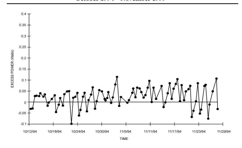
Excess Power For NRL Pd-B Rod (Cell C) (0.75 wt. % B, 2.5 x 2.5 cm, V=0.12 cm³) October 1994 – November 1994  $P_X(max) = 380 \text{ mW}$
