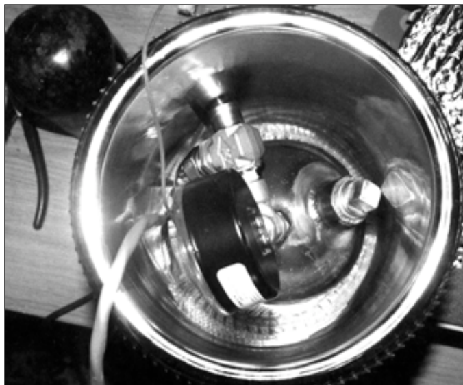
View inside dewar showing Case catalytic fusion cell mounted on resistance heater. NERL, Bow, NH. Photo: Ed Wall.
