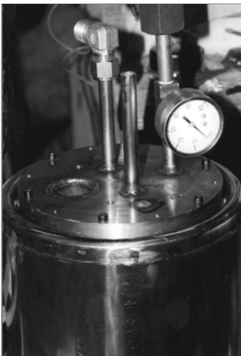
Dr. Case's large modified dewar cell, designed for catalyst beds up to one kilogram and aimed to achieve self-sustaining. Deuterium gas leaks are being fixed. Photo: Ed Wall.
