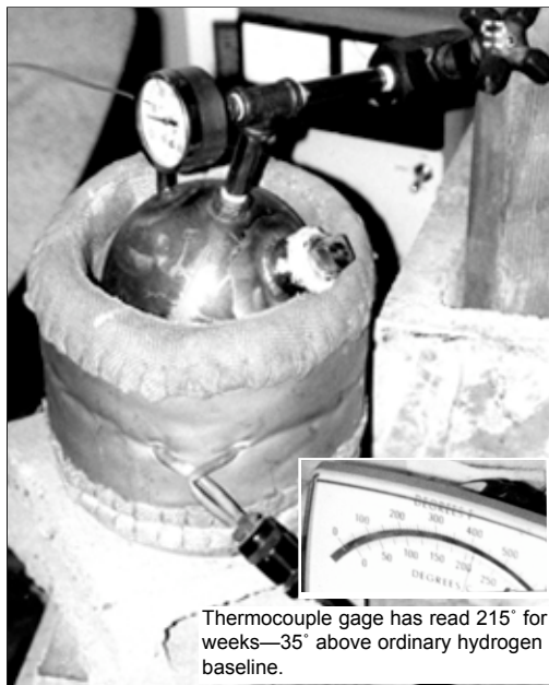
Catalytic fusion reactor in Dr. Les Case's lab, showing pressure gage and resistance heater collar. Photo: Ed Wall.
