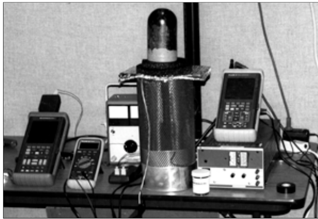
Small Case catalytic fusion cell (inside glass dewar, center) set-up for calorimetry calibration and “live” operation. Note: gas cylinder safety cap is used to secure thermal cover on dewar. NERL, Bow, New Hampshire.
