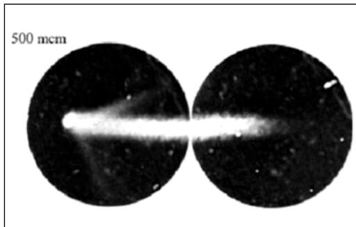
Figure 12. Comet-like marking with rays.
