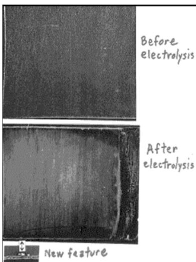
Figure 19. Trench on Ti cathode with sloshing on the sides.
