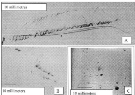
Figure 14. Markings on X-ray films set outside (A,B) and inside (C) vacuum chamber. Deuterium irradiation in glow discharge.
