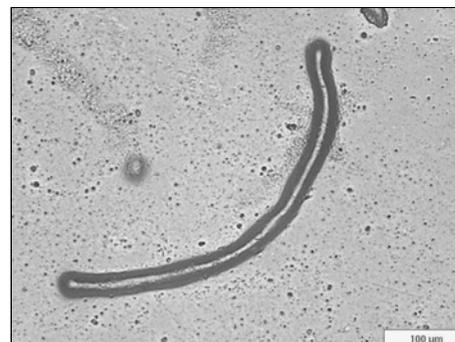
Figure 16. A trail marking on nuclear emulsion? From deuterium glow discharge experiment with W-W cathodes.
