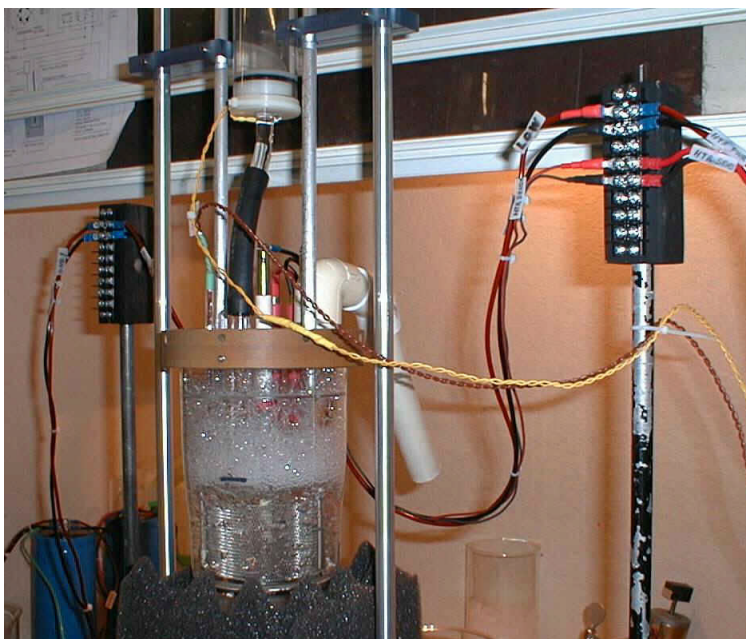
Figure 2. The photo of the setup showing the foam above the electrolyte. The dark cushion below the vessel helped to prevent bouncing of the scale. The inner diameter of the white PVC pipe was ~2 cm
