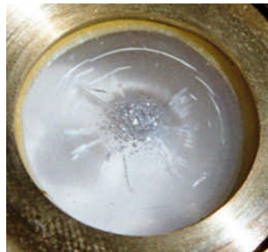
Fig.8. Photographs of post-effects upon Be window and the plastic window in the experiment with powerful X-ray laser beam generation.
