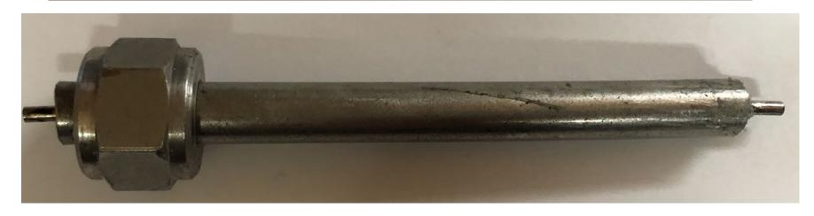
Codeposited Pd with PdBr<sub>2</sub> and LiBr on a 2mm diameter 10cm long Pd/Ag electrode
