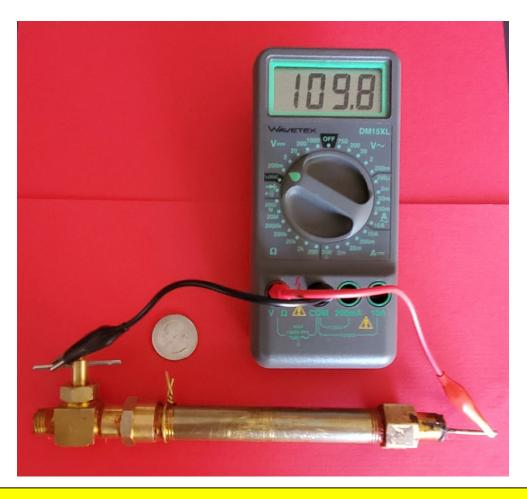
A LEC cell producing spontaneous and self-sustained electrical energy for several months into a DVM with a 10 M $\Omega$  input impedance
