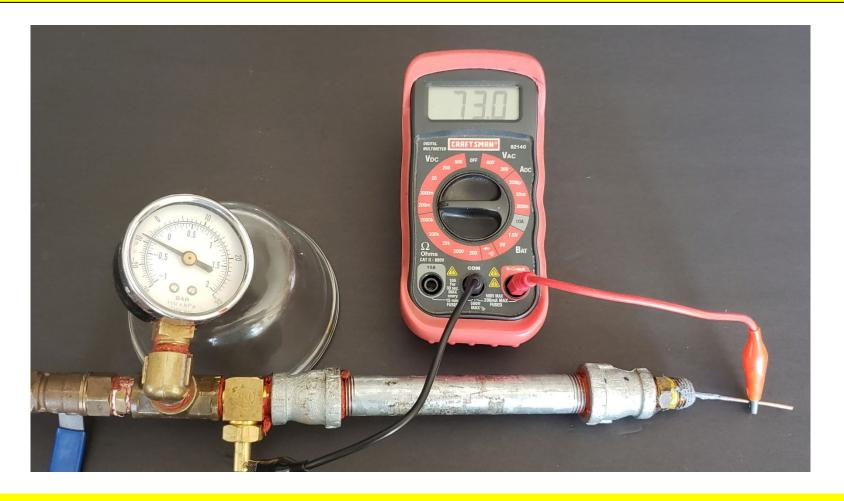
Another LEC cell producing spontaneous and self-sustained electrical energy for several months into a DVM with a 1  $M\Omega$  input impedance
