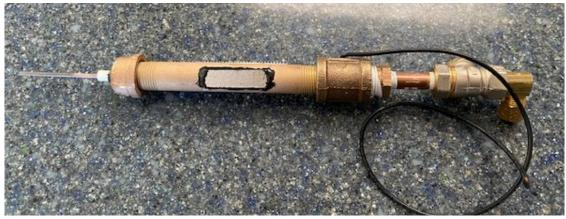
Mylar window to provide access for sensors to identify the ionizing radiation.
