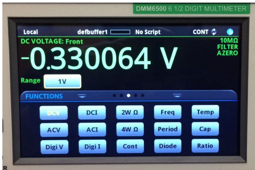
Figure 5 – Open circuit voltage measured on the brass - brass device after some time from the beginning of the tests.
