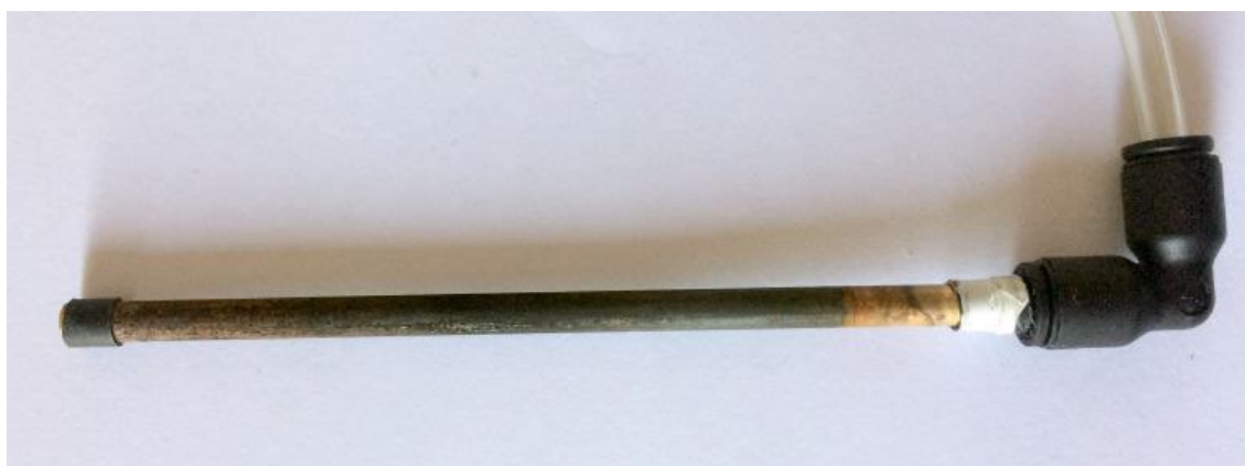
Figure 9 – Oxidation appearing on the WE after exposing to air (mainly left).
