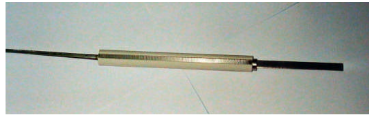
Figure 2. A ceramic holder with a heater and a planar sample
