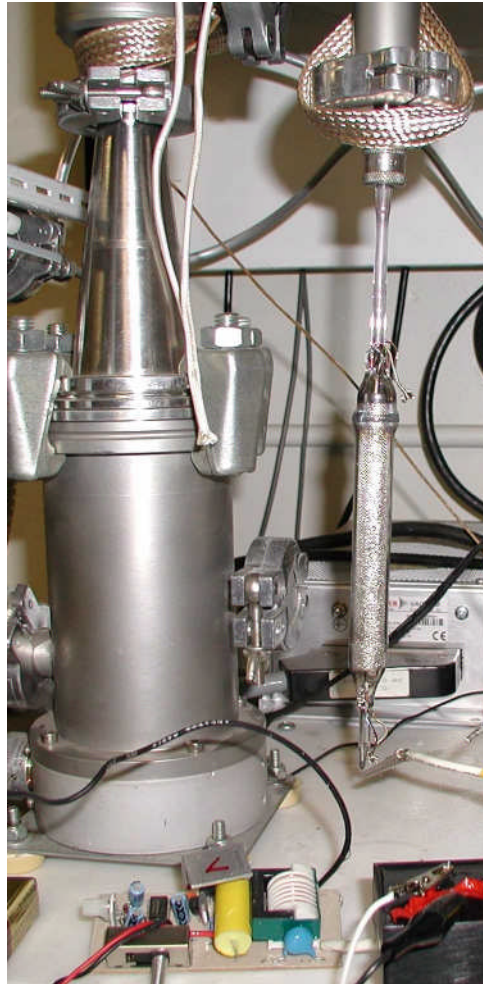
Fig. 10 Photo Of Sealed-Glass Type Glow Tube (Mounted On Vacuum Station)
