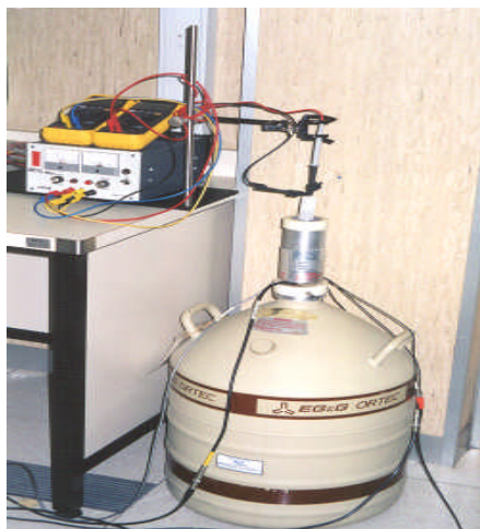
Fig.4 Cell over the detector
