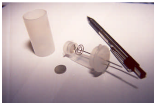
Fig.2 Detail of the thin film cathode and Pt contact
