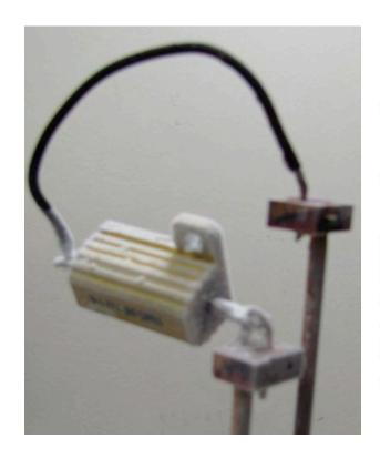
$1.008\Omega$  at 298K,  $0.988\Omega$  at 77K
