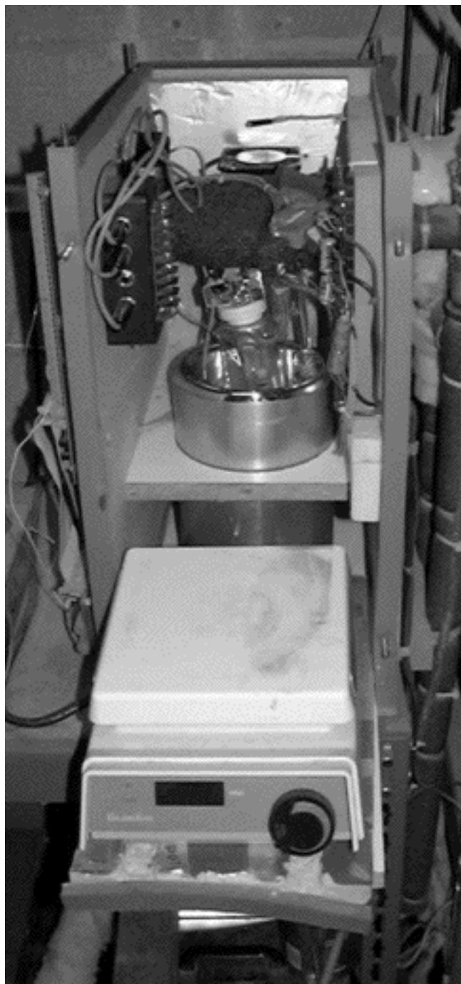
FIGURE 1. Picture of open flow-type calorimeter
