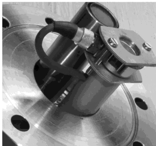
FIGURE 6. Si barrier detector (Ortec TB-016-050-1000) and GM tube (2.2-2.6 mg/cm 2 ).
