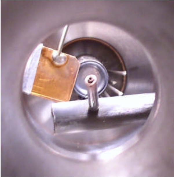
FIGURE 3. Cathode-eye view of the GM radiation detector. One of the copper absorbers is seen on the left. The anode is one of several designs using 2 mm wire covered by a glass insulator. The large tube from which it emerges is a glass-filled insulator.
