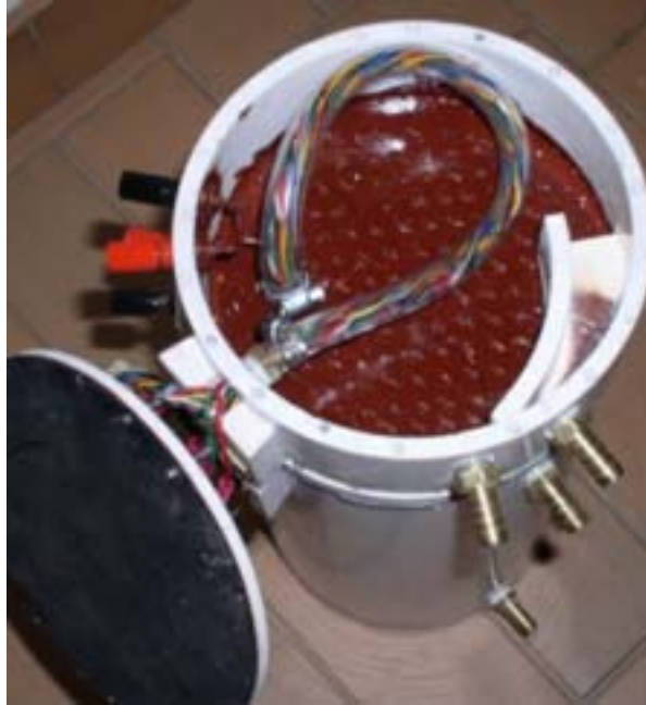
FIGURE 2. Interior of the lid showing the way in which water is caused to swirl, how the wires are passed through constant-temperature water, and the water-proof paint applied to the surface in which the thermocouples are located.
