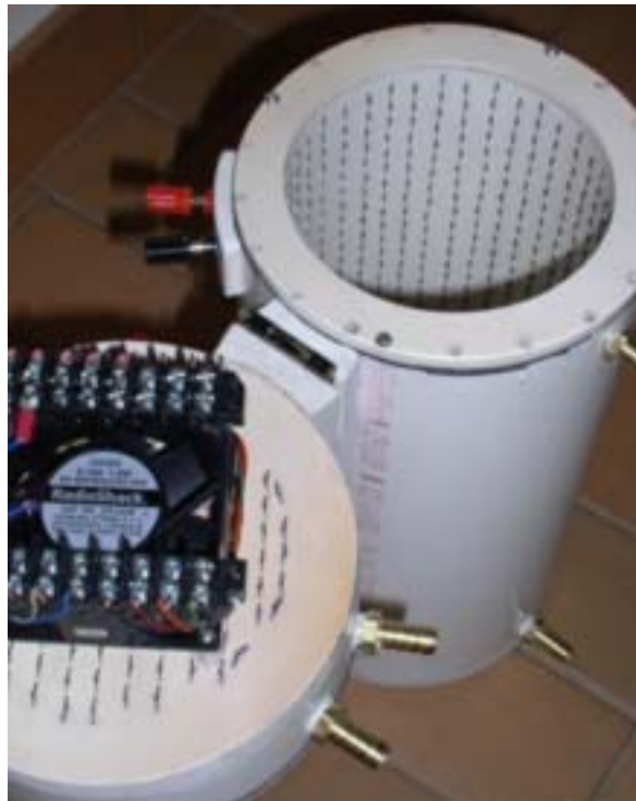
FIGURE 3. Interior of calorimeter shown with a fan attached to the lid. A fan at the bottom is not visible.
