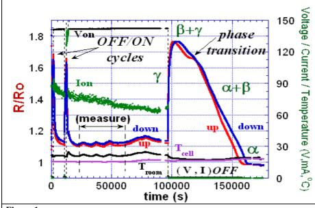
Figure 1. R/Ro data are meanly stable for a enough long time (from 30,000 to 90,000 seconds range)
