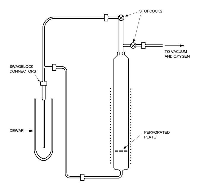
2. Schematic diagram of the apparatus employed for extracting carbon and nitrogen from cathodes previously used in electrolysis.
