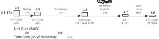
Total Emissions (g/kWh delivered): CO<sub>2</sub>: 358, NO<sub>2</sub>: 0.13
