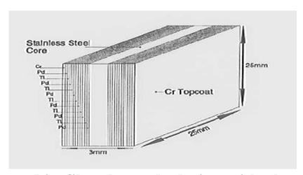
Early Multilayer thin-film electrode design with alternating layers of Pd & Ti with a topcoat of Cr ACS 233rd Annual Meeting,
