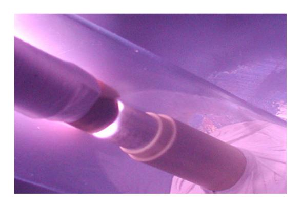
ACS 233rd Annual Meeting, Chicago, Il March 29, 2007 Typical result -- filtered AXUV detector indicates peak p=500 mTorr V=250V I=2A for a Pd cathode. The delay time of ~ msec before onset of x-raysis associate with D diffusion time. X-rays are > 600 eV with 250 V discharge! Blank experiment - a cu foil in front of the Be causes the trailing spike (x-rays) to disappear as expected,
