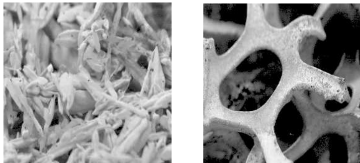
Figure 4. Auger Scan of Ni Microfelt (left) and Ni Foam (right) electrodes -White color indicates Pd-
