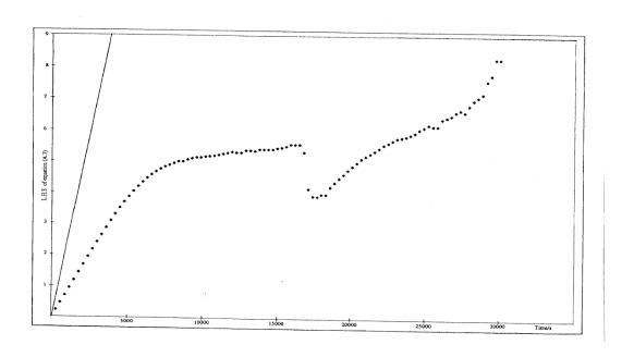
Fig. A.24 The analysis of the initial portion of the "cooling curve" shown in Fig. A.23 according to equation (A.3). The full line shows the R.H.S. of this equation plotted with  $C_PM = 28.3 \text{ JK}^{-1}$ ,  $(k_R')_{12} = 0.65 \times 10^{-9} \text{ WK}^{-4}$  and  $T_{bath} = 295.204 \text{ K}$ .
