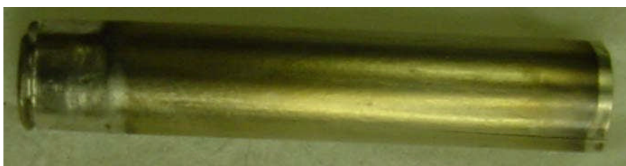
Figure 2 DS Cathode EAP2 after removal from the electrochemical cell.
