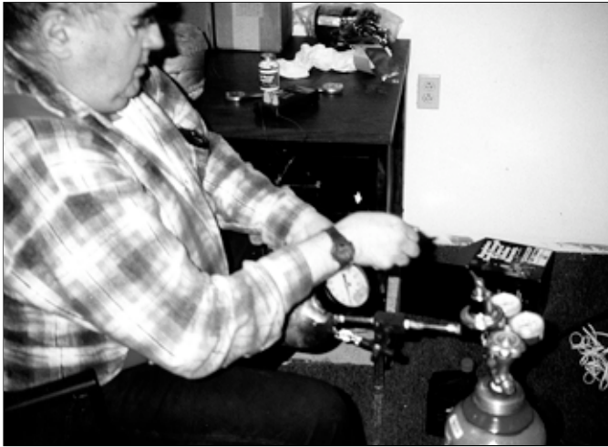
Dr. Les Case admits hydrogen gas from our H 2 tank via a pressure regulator into his prototype catalytic fusion reactor (April 30, 1998). Hydrogen cycling, heating, and evacuation of chemical reaction products is essential to conditioning the catalyst prior to admitting deuterium gas to the reactor. Then the excess temperature effect is seen. (Photo: E. Mallove)
