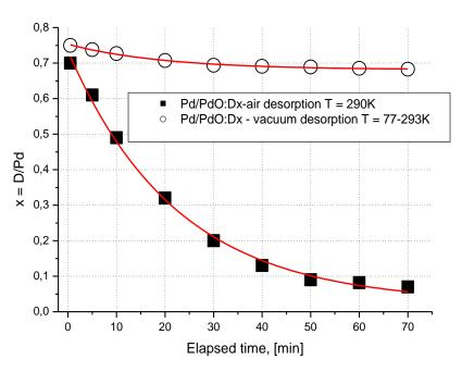
D-desorption rate from the Pd/PdO:Dx samples in vacuum (electrolysis at T=280 K with cooling down to T=77 K after electrolysis termination)) and in air at ambient conditions (electrolysis at T=290 K). Notice very low D-desorption rate in vacuum
