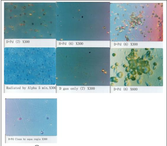
Fig. la shows the photo of CR-39 from the  $D_2$ +Pd cell. It is clear that there are some tracks of energetic charged particles. In order to estimate the energy and charge of these particles, we show the photo of CR-39 irradiated by a particle source (Am
