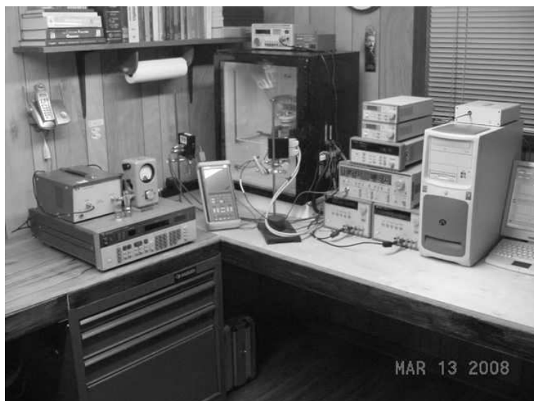
Figure 2. A typical equipment setup for this work; data is collected by a Labview-controlled Agilent 34970A and all data is displayed and stored on a PC.
