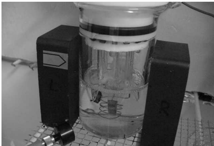
Figure 3. Typical cell configuration. Magnets as shown provide a 700 gauss field across the cathode face. In the foreground is the optical spectrometer detector used in tuning the lasers within 0.25 nm. Air is vigorously stirred within the temperature-controlled enclosure.
