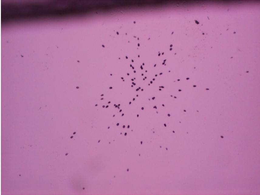
**Figure 4. Cluster of tracks produced during five hours of electrolysis. The area of 1000 by 1300 microns was photographed under a magnification of X40, after six hours of etching. The mean track density, over the area of 1 mm<sup>2</sup>, is about 11,000 tracks per cm<sup>2</sup>. This is three orders of magnitude higher than in the areas outside the four clusters, on the same CR-39 chip. A section of this photo, under a higher magnification, is shown in Figure 6.**
