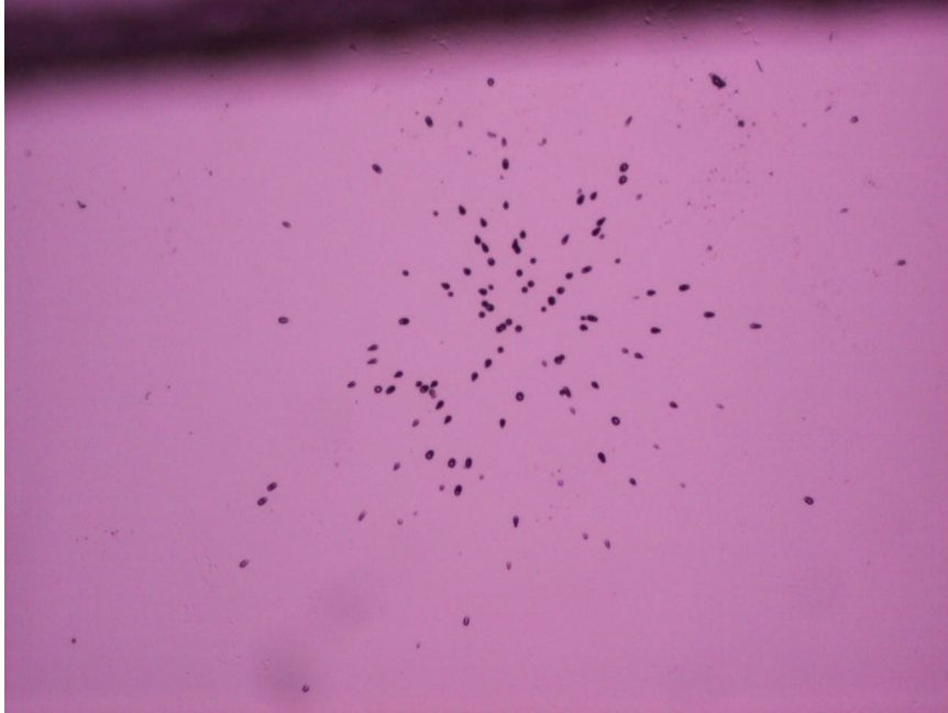
Figure 4. Cluster of tracks produced during five hours of electrolysis. The area of 1000 by 1300 microns was photographed under a magnification of X40, after six hours of etching. The mean track density, over the area of 1 mm 2 , is about 11,000 tracks per cm 2 . This is three orders of magnitude higher than in the areas outside the four clusters, on the same CR-39 chip. A section of this photo, under a higher magnification, is shown in Figure 6.
