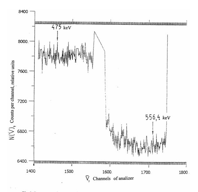
Fig.2. Instrumental spectra of gamma-quanta in the vicinity of the energies of identification of  $_{45}Rh^{102}$ : E=475.1 keV (38.4 quanta per 100 decays) and E=556.41 keV (96 quanta per 100 decays)
