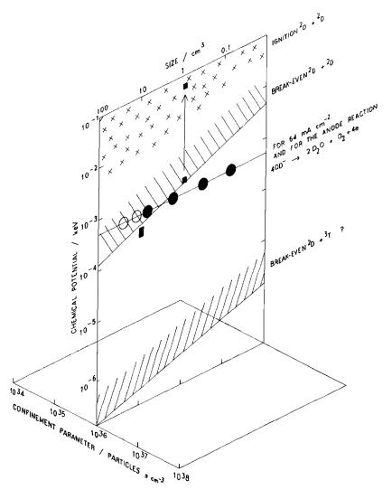
Fig. 2. Confinement parameter-chemical potential-size diagram for <sup>2</sup>D+ <sup>2</sup>D fusion reaction in Pd cathodes; projection to the <sup>2</sup>D+<sup>3</sup>T reaction. Open circles: systems currently being investigated.
