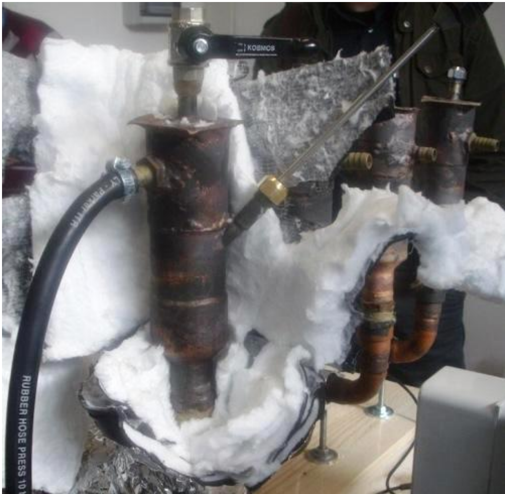
Figure 4 showing the chimney with the black outlet tubing, the thermocouple holder and on the top, the steam exhaust valve. (Photo: Giuseppe Levi).
