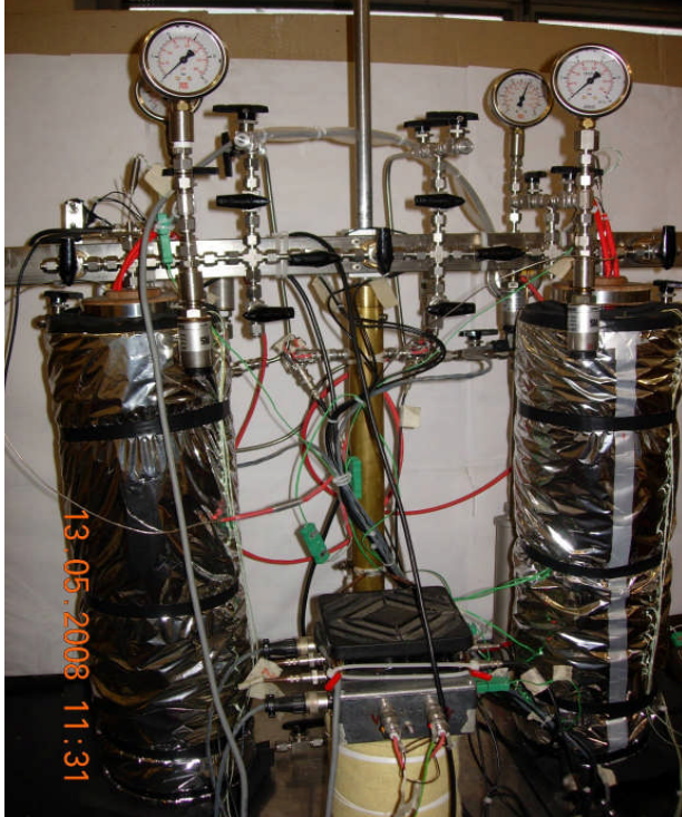
Figure 1. The twin chamber differential reactor developed at INFN-LNF. Pressure: up to 100 bar. Temperature: up to 320°C. Useful volume of the crucibles: 15 cm 3 .
