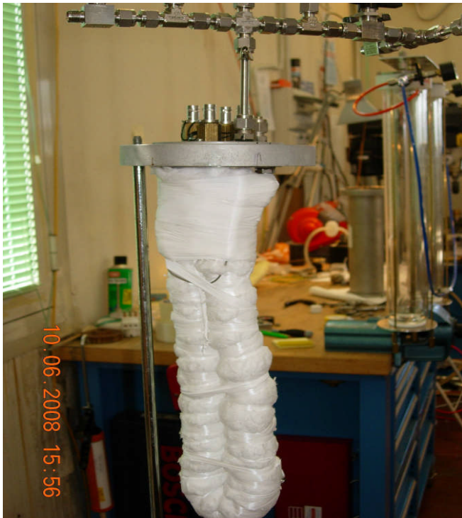
Figure 3. The braid placed inside thermal insulation.
