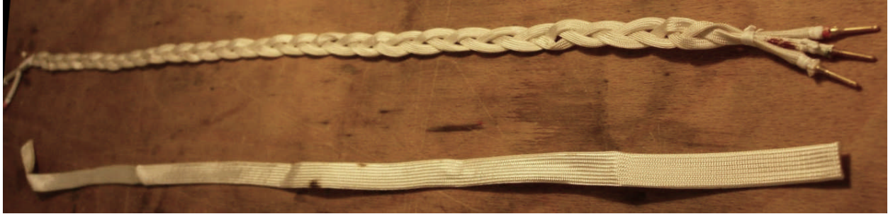
Figure 2. Three wires braided together: 1 coated Pd wire and 2 Pt wires ( Pt_{cal} , Pt_{mon} ). Each wire is 50\mu\text{m} in diameter. The diameter of the fibre-glass sheaths is 2 mm. The braid is completely covered inside a larger sheath (6 mm) shown below. Ultra-pure ( >99.99\% ) Pt was used for Pt_{cal} and Pt_{mon} . Pt_{cal} serves as a calibration Joule heater and Pt_{mon} serves as a distributed thermometer.
