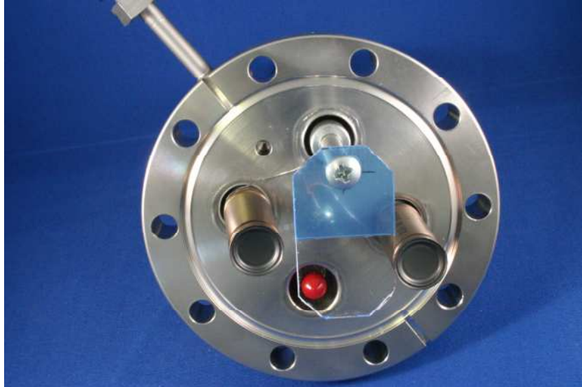
Figure 4 – Detector end-plate configured with dual GM tubes and plastic absorber. (CR-39 is used here as a 100mg/cm 2 absorber.)
