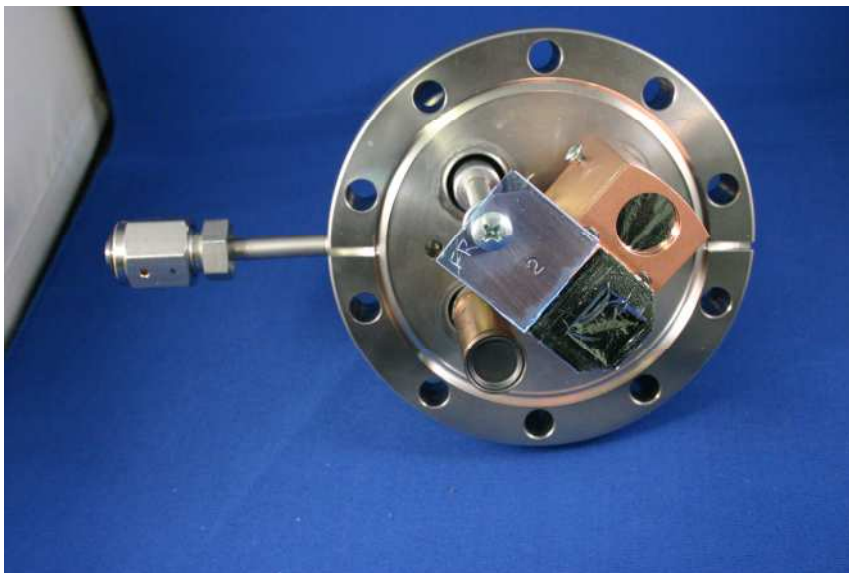
Figure 5 – Detector end-plate configured with 2mg/cm 2 GM tube, Si detector, 1.8 micron aluminum absorber and CR-39 detector.
