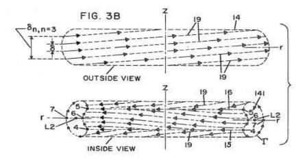
For **topological stability** of field-line configuration in external **vacuum**, it is ESSENTIAL (according to physical doctrine of "line-tying") that EVERY field line in the external vacuum should **cut** a current-carrying conductor at an angle <u>other</u> than perpendicular!
